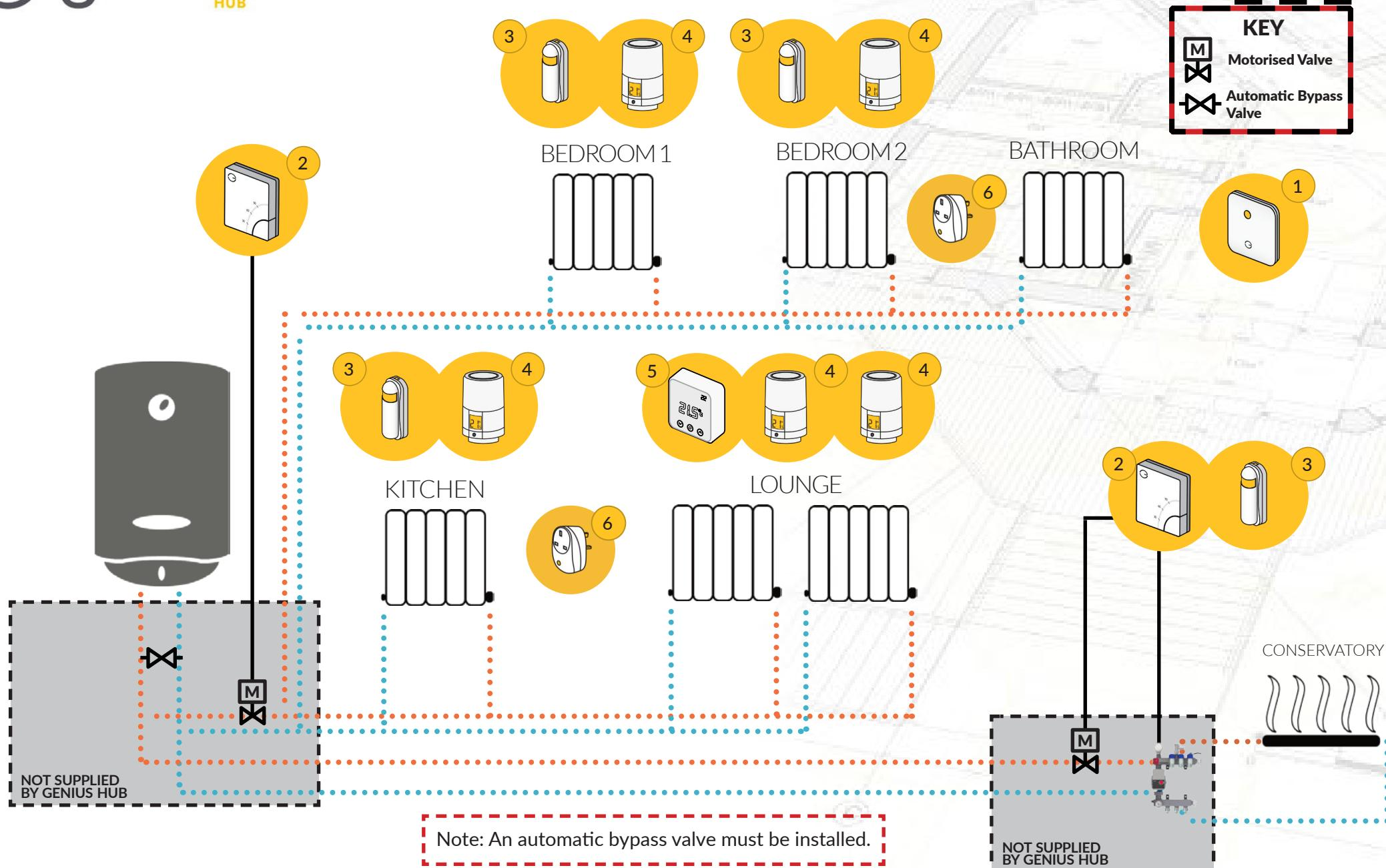
1 - Genius Hub | 2 - Electric Switch | 3 - Room Sensor | 4 - Radiator Valve | 5 - Room Thermostat | 6 - Smart Plug
